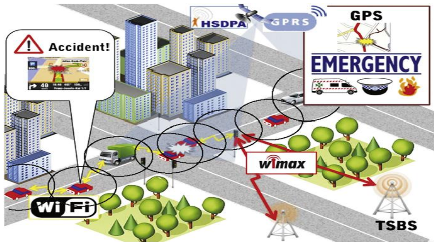
Fig. 1 Typical urban VANET scenario Circles represent the Wi-Fi coverage of vehicles.
